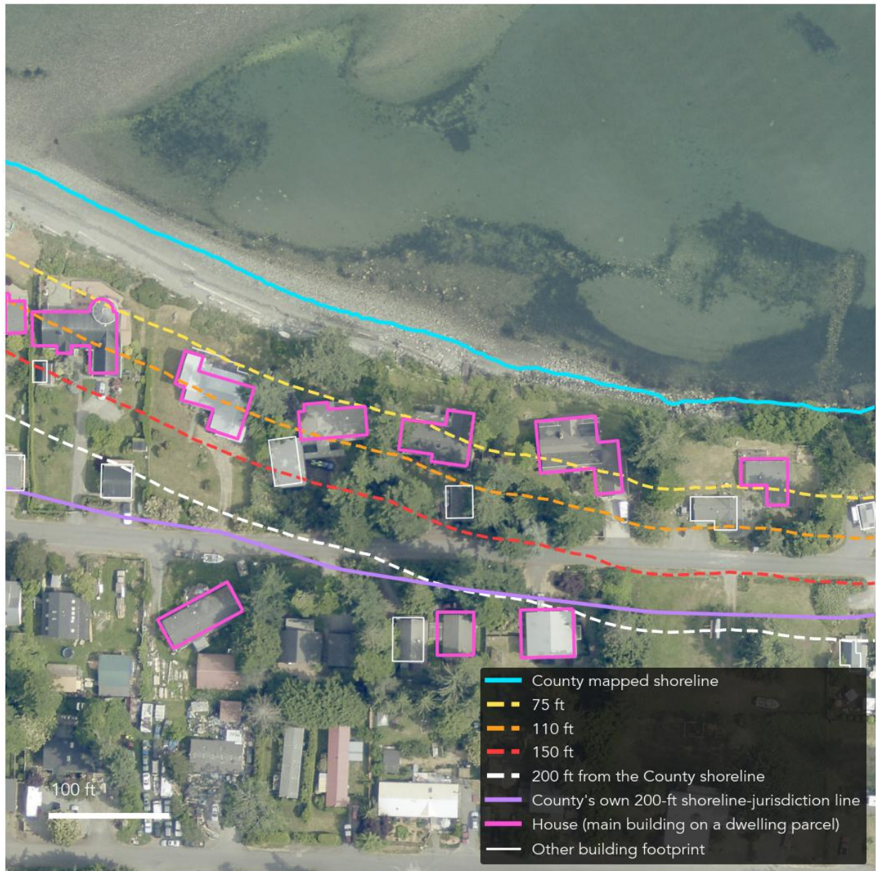
Figure 2. The method on one stretch of shoreline. County 2025 aerial imagery. The County's mapped shoreline (cyan) follows the water's edge, seaward of the beach and the vegetation line, so distances measured from it are longer than distances from the high-water line and the counts are conservative. The white dashed line is 200 ft from that shoreline; the purple line is the County's own 200-ft line, which here sits farther inland on the left and closer on the right. Some buildings visible in the imagery have no County footprint and are not counted.
